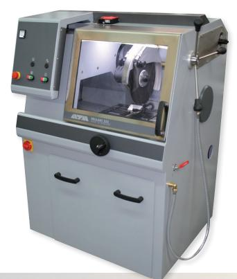
The universal wet abrasive cut off machine BRILLANT 255 with manual travel and fine dynamic cuting allows precise, soft touch cutting with 2 axes in arbitrary directions (Y/X axis) and can be equipped with a manual Z-axis for parallel serial cuts (option). Side openings allow cutting continuous long parts in the spacious cutting chamber of this solid and powder-coated aluminium construction.
